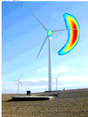
Figure 1: Picture of test set-up for acoustic measurements on the GAMESA baseline turbine. The distribution of noise sources in the rotor plane is projected onto the picture. The rotor rotates clockwise
